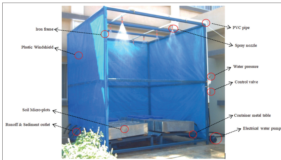
Figure 1: General view of rainfall simulator used in this study
