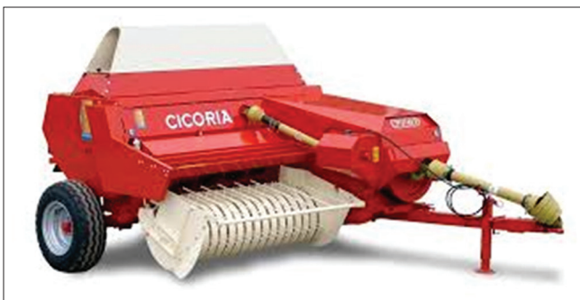
Figure 1: Small rectangular baler type (Ćicoria 454)
