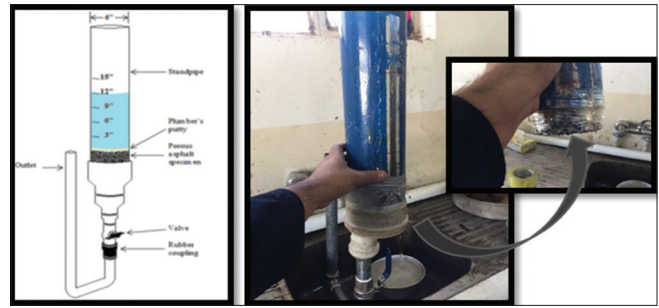
Figure 5: Permeability test schematic
