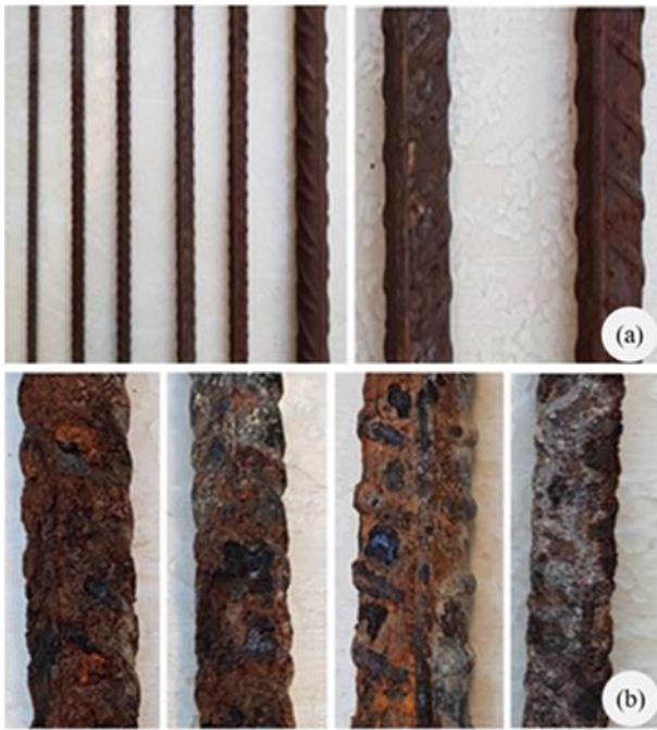
Fig.4. (a) Specimens exposed to natural atmosphere for 5 years, (b) different corrosion products appeared in SL group.
