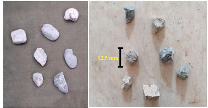
Fig. 4: Materials used in CAA tests. A) Normal aggregate particles, B) Harsh aggregate particles
