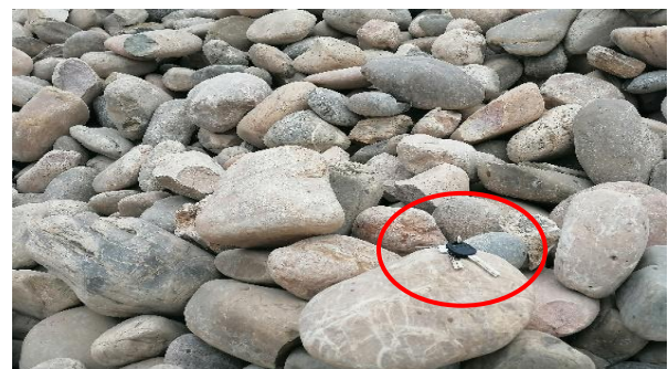
Fig. 2. Bolder diameter more than 3 inches
