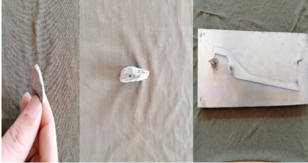
Fig. 6. Proportional caliper Apparatus to identify flat and elongated particles
