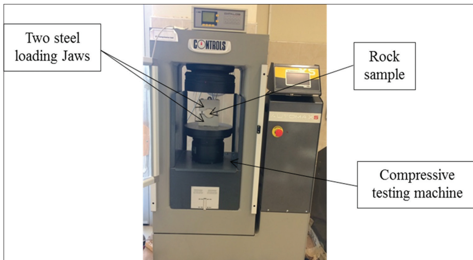
Figure 2: Compressive testing machine with two steel loading jaws to perform Brazilian tensile strength
