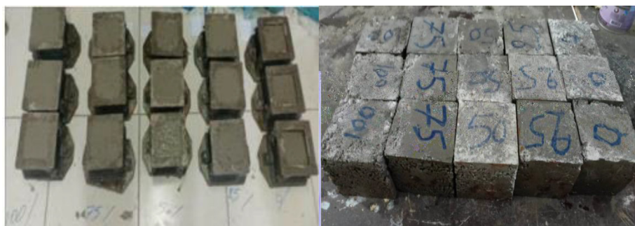
Figure 6. Concrete cubes measuring 10 × 10 × 10 cm with limestone and marl aggregate mix.
