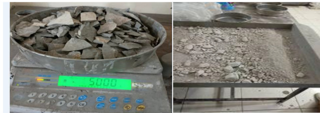
(c)Marl aggregate before abrasion. (d)Marl aggregate after abrasion.
