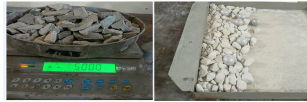
(a)limestone aggregate before abrasion. (b)limestone aggregate after abrasion.
