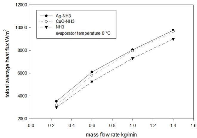
Figure 3 (b) Average heat flux at saturation temperature 0 °C
