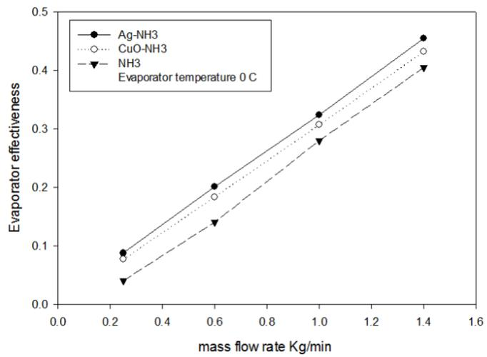
Figure 5 (b) Effectiveness of various nanofluids at different flow rates and evaporator temperature of 0° C.
