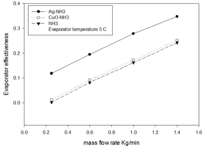
Figure 5 (a) Effectiveness of various nanofluids at different flow rates and evaporator temperature of 5° C
