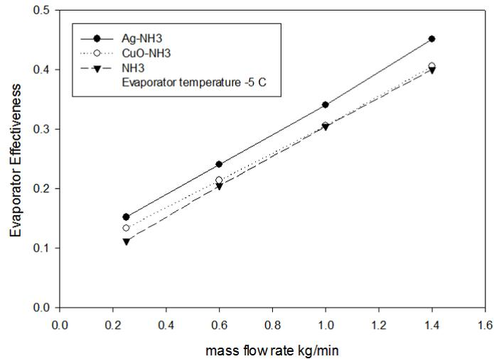
*Figure 5 (c) Effectiveness of various nanofluids at different flow rates and evaporator temperature of  $-5^{\circ}\text{C}$*
