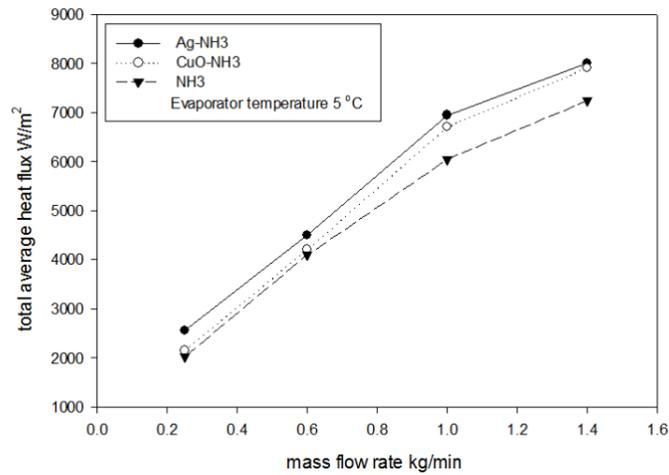
Figure 3 (a) Average heat flux at saturation temperature 5 °C
