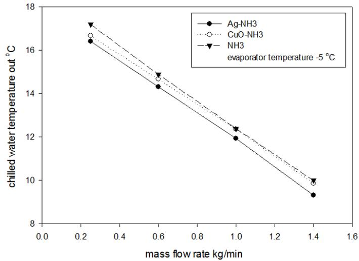
Figure 4 (c) Average outlet water temperatures at evaporator temperature -5°
