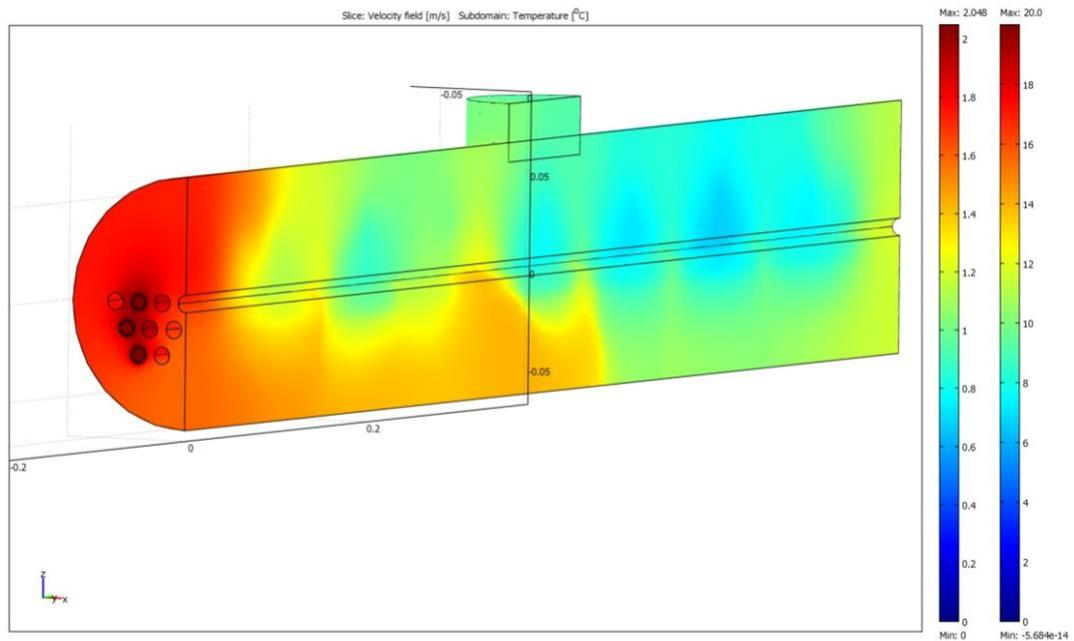
Figure 2 Temperature profile distribution in the shell of the heat exchanger.
