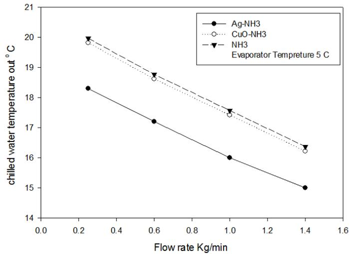
Figure 4 (a) Average outlet water temperatures at evaporator temperature 5° C
