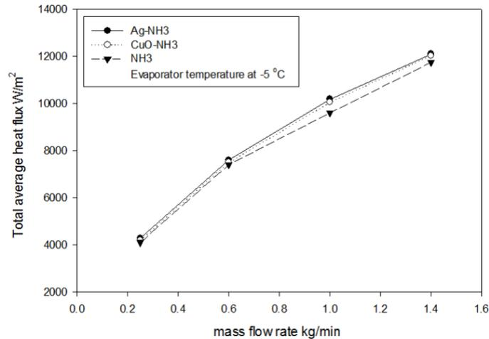
Figure 3 (c) Average heat flux at saturation temperature  $-5^{\circ}C$
