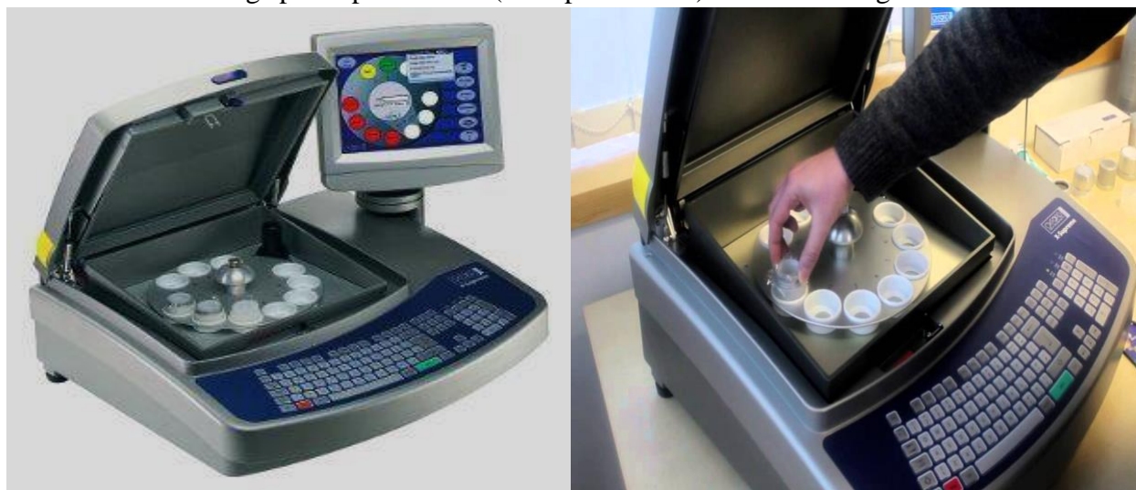
Figure 5. Illustrates the XRF analysis (X-ray fluorescence) by spectrometer X-Supreme8000
